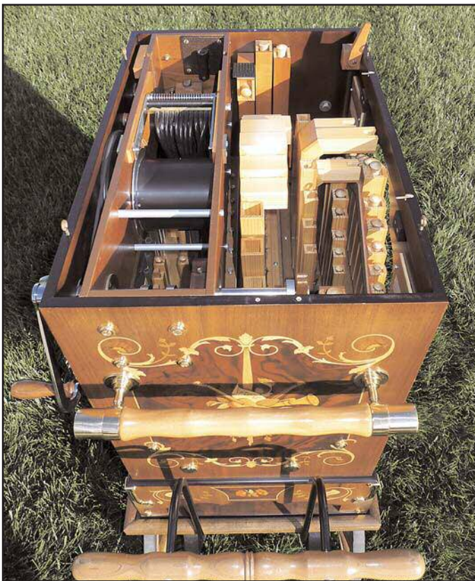
Figure 6. A good view of the melody registers, accompaniment pipes and roll frame.
