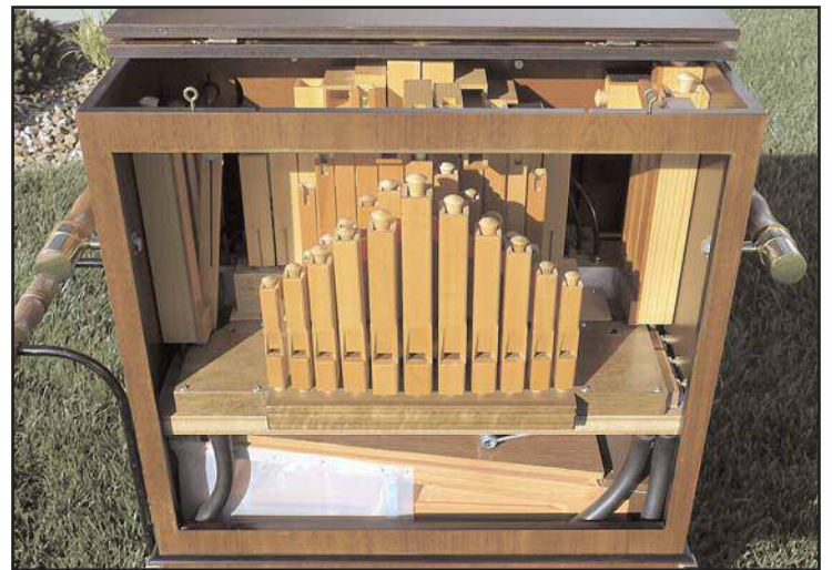
Figure 7. A front view with façade removed. Notice the bellows, 11 concert flutes and the accompaniment pipes (three on the left and three on the right).
