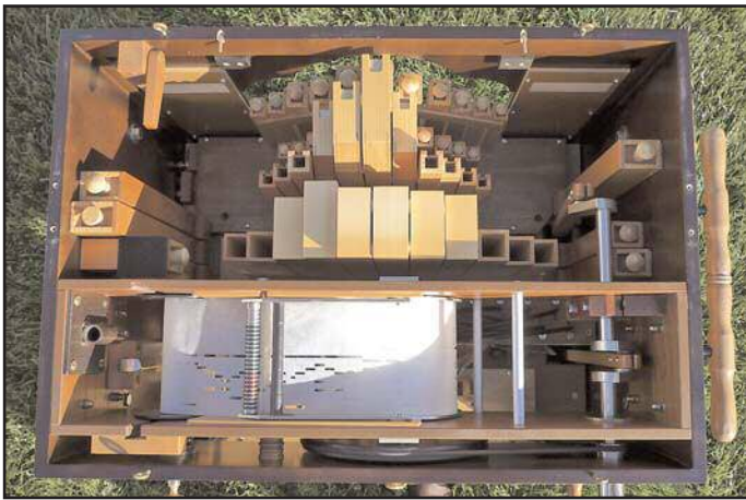
Figure 4. A top view of 20/78 case without the cover. There are good views of melody and accompaniment pipes as well as the crank handle with twin cams to the lower bellows.
