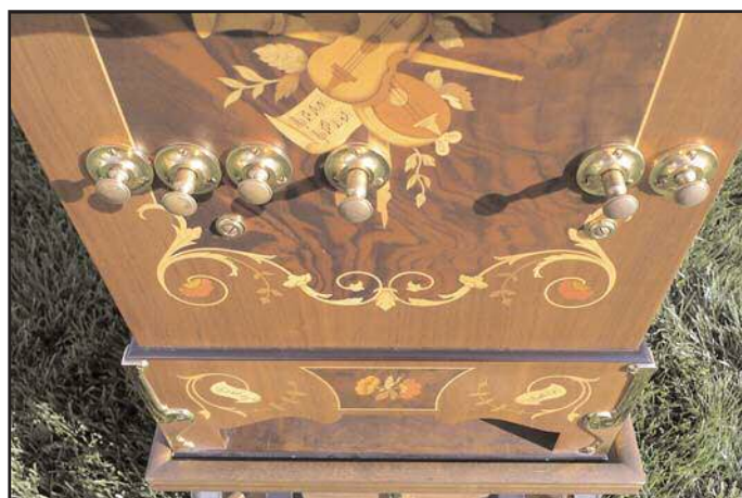
Figure 3. A view of the brass on/off stops for the six melody registers.
