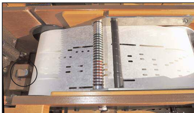
Figure 10. A view of the tracker bar with the standard 20-note roll in place. The volume control lever (pressure regulator) is just left of the roll (circled in photo).
